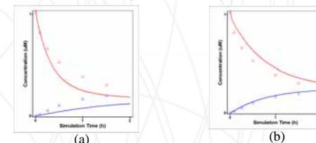
**Figure 4.** Predicted (lines) and *in vitro* (squares) concentration-time profiles after apical administration of 1 µM propranolol in the presence of 100 nm bafilomycin. (a) lysosomal pH set to be 4. (b) lysosomal pH set to be 5.5. Simulated apical, basolateral concentrations are shown in red and blue, respectively. A similar match between simulated and observed profiles was obtained for basolateral administration (data not shown).
